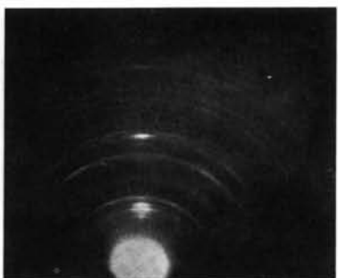
Fig. 7. Zn, {001} and {100}, possibly associated with rapid deposition.
