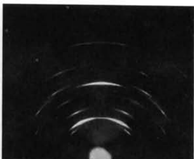
Fig. 8. Zn, {112} on NaCl cleavage face.
